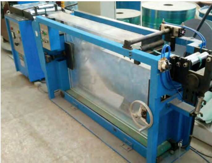
Accumulator of tape armoring
